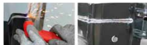
STEEL: 6 mm max ALU: 4 mm max (Speed = 20 cm /min at 20A)
